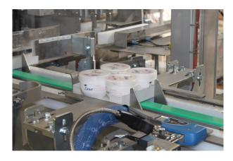
Unilever's Dubai site is the largest personal care factory in the Middle East and Africa, producing hair and skincare products. There, Gebo Cermex has recently supplied a complete end-of-line solution, including one piece of the company's spearhead equipment, the WB46 wrap-around case packer, a smart "Industry 4.0" system designed for greater flexibility, hygiene, and ergonomics.
